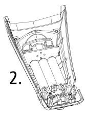
2. Remove the old batteries and/or insert a new set of alkaline batteries. Pay attention to the orientation of the batteries and follow the drawing in the torch.
