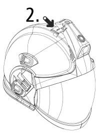
Attaching the torch: Allow the helmet torch to slot into place at the front first (1) and then at the back to match the mounting bracket on the helmet (2). Press firmly on the mounting bracket and make sure that the torch is fixed in place.
