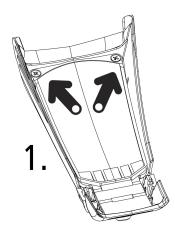
1.Unscrew the screws that hold in place the housing cover.
