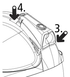
Place first the head of the torch on the frontal part of the helmet ridge so it fits the shape of the frontal plate (3). Then bring down the tail of the torch to the helmet ridge so the adhesive adheres to the surface (4). Make sure that you put enough pressure with your hands on the tail of the torch so the mounting bracket sticks well on the helmet surface. Make sure the helmet torch is fixed in place.
