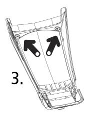
3. Reassemble the torch and tighten the screws on the housing. Check that the housing cover is properly positioned and that the screws are tightened.
