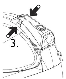
Detaching the torch: Press firmly and simultaneously on the buttons on the tail of the torch (3) and remove the torch.
