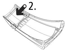
Clean well the helmet surface (1) with 90% ethanol alcohol and then remove the adhesive protective tape from the mounting bracket of the torch (2).
